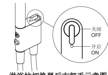
淋浴柱切换器后方把手示意图 The handle behind the column
